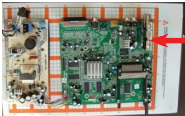
EMScanner spatial scan at 50MHz with noise injection at right edge of board.
